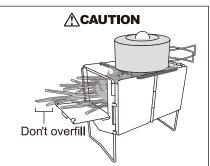
Do NOT overfill past the doorways. May result in incomplete combustion and increased smoke. May also cause the fire pit to tip over.
