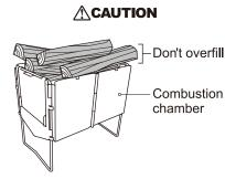
Do NOT overfill beyond the top of the combustion chamber. May result in incomplete combustion and increased smoke.
